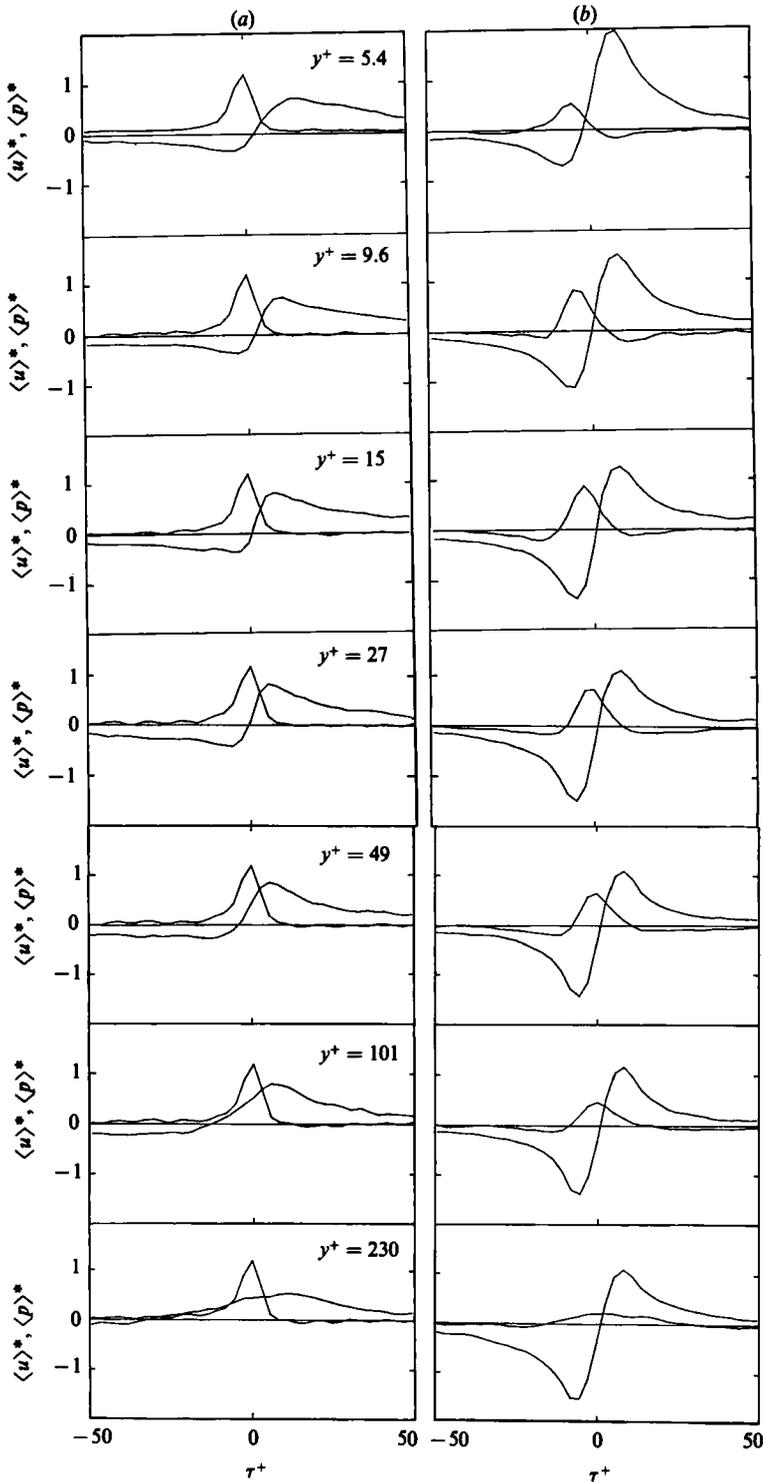
FIGURE 14. Conditional averages of  $p_w$  and  $u$  at various  $y^+$  positions in the spot for (a) detection of positive pressure peaks ( $k = 2.5$ ), and (b) VITA detection of accelerating events ( $K = 1.0$ ,  $T^+ = 22$ ).  $\langle u \rangle^* = \langle u \rangle / u_{rms}$ , and  $\langle p \rangle^* = \langle p \rangle / k p_{rms}$  in (a) and  $\langle p \rangle / p_{rms}$  in (b).  $\tau^+$  denotes time, in wall units, relative to the detection time.  $x = 1.54$  m.
