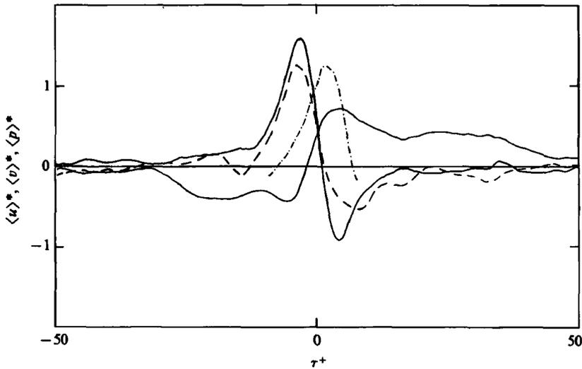
FIGURE 8. Aligned (two iterations) conditional averages of  $p_w$  (dashed curve), and  $u$  and  $v$  at  $y^+ = 15$  for VITA detection of decelerating events in the  $v$  signal ( $K = 2$ ,  $T^+ = 12$ ). -.-.-, pressure pattern shifted in time to correct for the streamwise separation between the hot wire and the pressure transducer.
