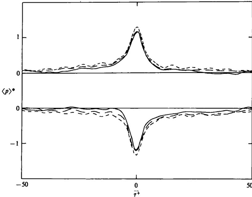
FIGURE 3. Conditional averages of  $p_w$  for positive and negative pressure-peak events (—,  $k = 1.5$ ; --,  $k = 2.5$ ; - · -,  $k = 3.5$ ) in a turbulent boundary layer ( $x = 4$  m,  $U_\infty = 10.2$  m/s).
