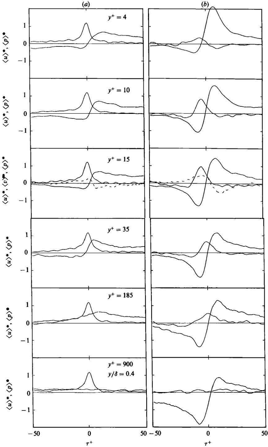
FIGURE 5. Conditional averages of  $p_w$  and  $u$  at various  $y^+$  positions, and  $v$  (---) at  $y^+ = 15$ , for (a) detection of positive pressure peaks ( $k = 2.5$ ), and (b) VITA detection of accelerating events ( $k = 1.0$ ,  $T^+ = 24$ ).  $\langle u \rangle^* = \langle u \rangle / u_{rms}$ , and  $\langle p \rangle^* = \langle p \rangle / kp_{rms}$  in (a) and  $\langle p \rangle / p_{rms}$  in (b).  $\tau^+$  denotes time, in wall units, relative to the detection time.  $x = 4$  m.
