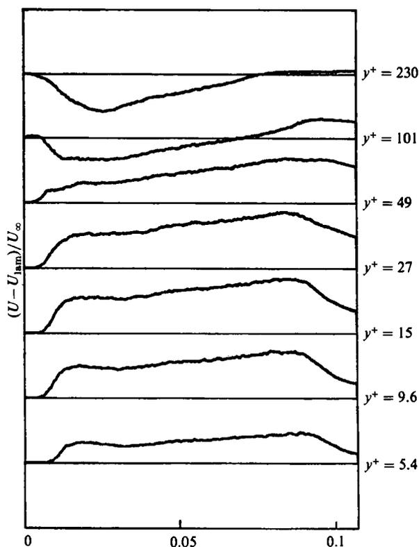
FIGURE 12. Ensemble-averaged velocity signatures of the spot at various distances from the wall (averaged over 500 realizations).  $U_\infty = 10.1$  m/s,  $x = 1.54$  m. The distance between horizontal lines corresponds to 0.5.
