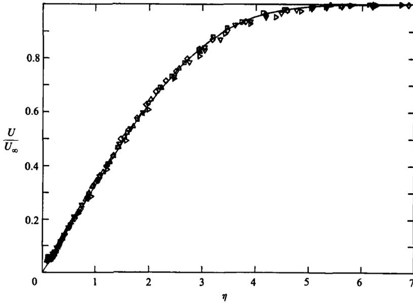
FIGURE 2. Laminar boundary-layer profiles for  $U_\infty = 10$  m/s and various positions along the plate, plotted in similarity coordinates ( $\eta = y(U_\infty/\nu x)^{1/2}$ ). Virtual origin of boundary layer at  $x = -0.03$  m. —, Blasius profile;  $\square$ ,  $x = 0.28$  m;  $\diamond$ ,  $x = 0.55$  m;  $\triangle$ ,  $x = 0.80$  m;  $\nabla$ ,  $x = 1.05$  m;  $\triangleright$ ,  $x = 1.54$  m.
