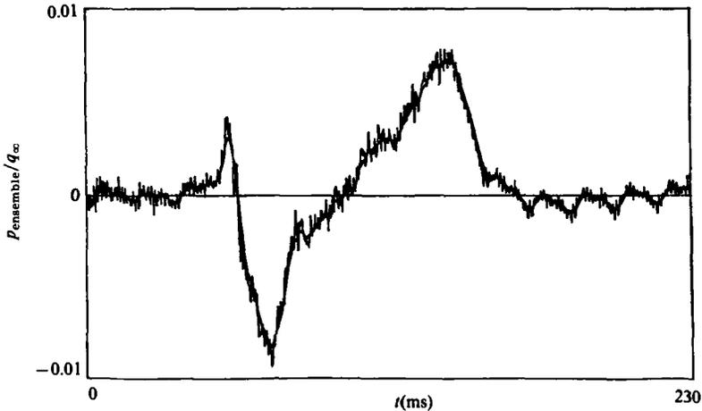
FIGURE 11. Ensemble-averaged pressure signature of 500 spots, and its low-pass filtered counterpart.  $x = 1.54$  m,  $x_{\text{trig}} = 0.29$  m,  $U_{\infty} = 10.1$  m/s.  $t$  is delayed 0.090 s from instant of triggering.
