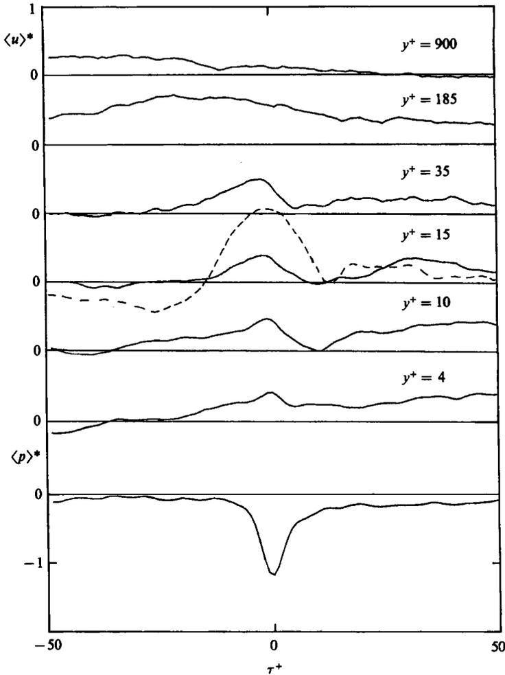
FIGURE 9. Conditional averages of  $p_w$ , and  $u$  at various distances from the wall for detection of negative pressure peaks ( $k = 2.5$ ). Aligned  $u$  pattern (---) at  $y^+ = 15$  is also included.
