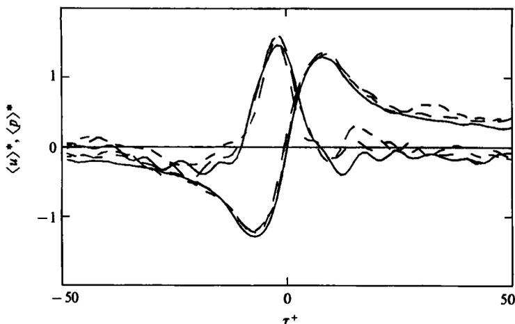
FIGURE 7. Aligned (two iterations) conditional averages of  $p_w$ , and  $u$  at  $y^+ = 15$  for VITA detection with various threshold levels, —,  $K = 1.0$ ; --,  $K = 1.5$ ; - · -,  $K = 2.0$ .  $T^+ = 24$ . Note that the  $u$ - and  $p$ -averages here have been normalized with  $K^{\frac{1}{2}}$  times the respective r.m.s. value.
