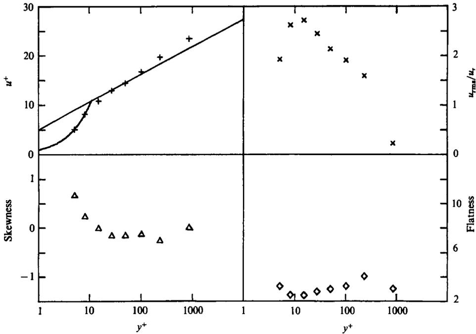
FIGURE 13. Profiles of mean velocity, streamwise turbulence intensity, skewness and flatness in the interior of the spot.  $x = 1.54$  m. Straight line in mean velocity plot represents  $u^+ = (1/0.41) \ln y^+ + 5.0$ .
