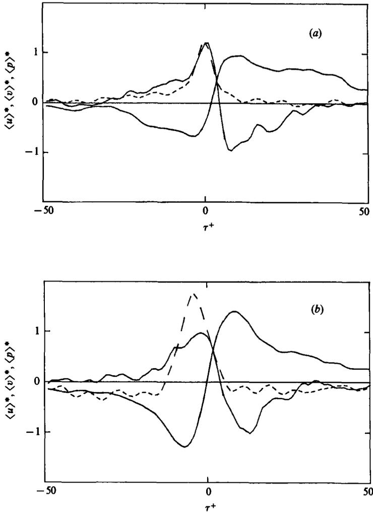
FIGURE 6. Aligned (two iterations) conditional averages of  $p_w$  (dashed line) and  $u$  and  $v$  at  $y^+ = 15$ . (a) detection of positive pressure peaks ( $k = 2.5$ ), (b) VITA detection of accelerating events ( $K = 1$ ,  $T^+ = 24$ ).  $x = 4$  m.
