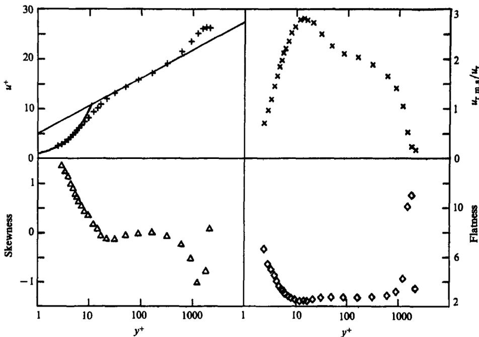
FIGURE 1. Profiles of mean velocity, streamwise turbulence intensity, skewness and flatness in a turbulent boundary layer.  $U_\infty = 10.2$  m/s,  $x = 4.0$  m. Straight line in mean velocity plot represents  $u^+ = (1/0.41) \ln y^+ + 5.0$ .
