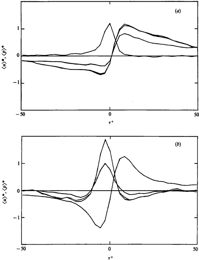
FIGURE 15. Conditional averages of  $p_w$  and  $u$  at  $y^+ = 15$ , for zeroth, first and second iteration in the alignment procedure. (a) Alignment of  $u$  for positive pressure-peak events ( $k = 2.5$ ). (b) Alignment of  $p$  for accelerating VITA events ( $K = 1.0$ ,  $T = 22$ ).
